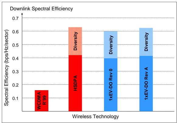
Figure 14: Comparison of Downlink Spectral Efficiency<sup>43</sup>
