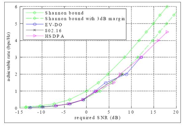
Figure 16: Performance Relative to Theoretical Limits<sup>45</sup>
