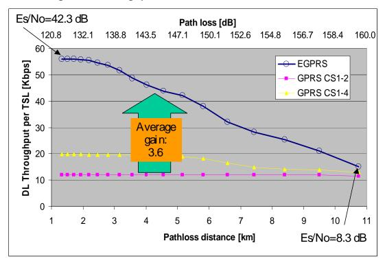
Figure 4: Throughput versus Distance for EGPRS/EDGE<sup>29</sup>
