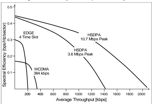
Figure 13: GSM Family Downlink Spectral Efficiency<sup>42</sup>
