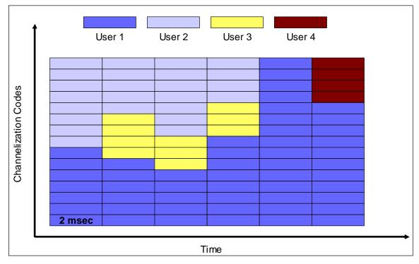
Figure 8: High Speed – Downlink Shared Channels (Example)
