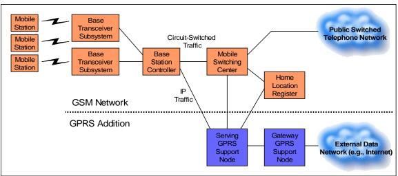
Figure 2: GSM/GPRS Architecture
