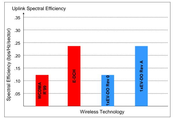
Figure 15: Comparison of Uplink Spectral Efficiency for Different Technologies<sup>44</sup>
