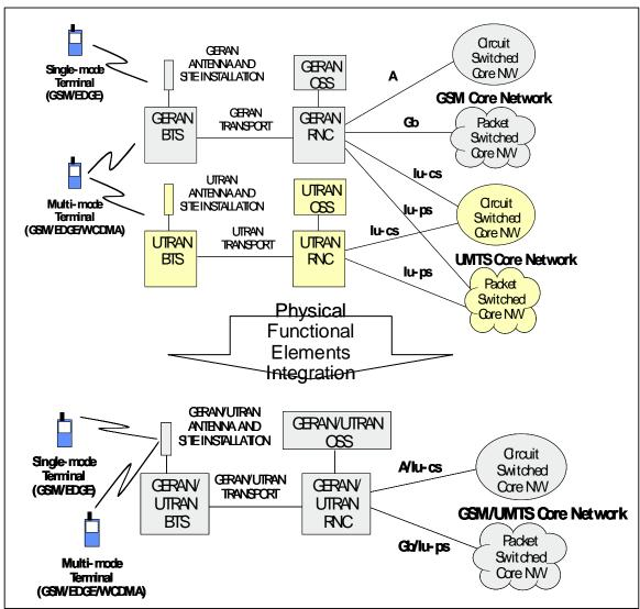
Figure 11: Integration of UMTS and GSM/EDGE Core Network Equipment<sup>39</sup>
