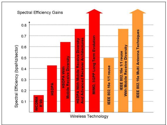
Figure 17: Enhancements in Spectral Efficiency of 3GPP Systems and WiMAX<sup>46</sup>
