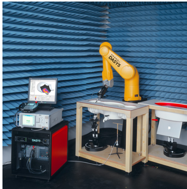
Figure 1: DASYS52 NEO dosimetric assessment system with SAM and elliptical flat phantoms for SAR assessments according to [1].
