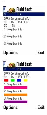
**Red**: Current ARFCN carrying the serving cell's BCCH or PBCCH (if PCCCH used in cell), in GPRS-idle mode. Displays 'xxxxx' when GPRS-detached. If in dedicated mode, this displays the current ARFCN used, and may slowly rotate through the hopping sequence if hopping is used. Similarly, if a TBF exists, this may display the ARFCN used for the current TBF. [GSM 05.05:2.x]
