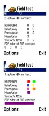
**Red**: The NSAPI (Network SAPI) used for the PDP context, in decimal. The SNDCP protocol uses the NSAPI to track and multiplex connections. The SAPI is a 4-bit value from 0-15. The meaning of the values are:
