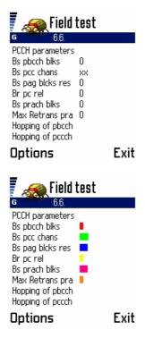
**Red**: BS\_PBCCH\_BLKS parameter, in decimal. This is a 2-bit value broadcast on the PBCCH (in PSI1) to indicate the number of blocks in the PDCH carrying the PBCCH. Values are from 0-3, which is 1 less then the actual number of blocks (i.e. 0 means 1 block, 1 means 2 blocks, etc). [GSM 04.60:12.25]
