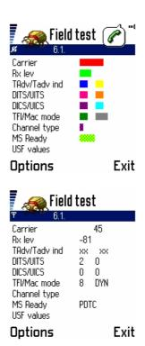
**Red**: The current ARFCN used for transmission/reception. If hopping is used, a 'H' is displayed in front of the channel. In idle mode, provided the MS is both IMSI and GPRS attached, this will be the same value as in Test 1.1. This value is not displayed (appears as 'x's) when not GPRS attached. [GSM 05.02]
