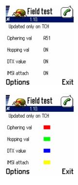
**Red**: Ciphering algorithm for Circuit Switched Connection. Can be A53, A52, A51 or "OFF". This value is only displayed when the phone is communicating with the network (on a TCH), when idle this value is displayed as "OFF". See Test 12.
