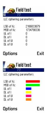
**Red**: The least significant 32-bits (i.e. bits 0-31) of the Kc, represented in decimal. The Kc is the 64-bit temporary key derived from the Ki and RAND parameter sent by the network used to cipher the GPRS traffic. The Kc and authentication works much the same way as it does for non-GPRS traffic, except it is over a higher level protocol. [GSM 03.60:6.8.1]
