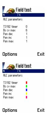
**Red**: Initial value of the T3192 timer. This timer controls how long the MS will wait after the end of the TBF (i.e. after the final ACK) before releasing the resources. This timer is aborted if the network assigns additional downlink resources or changes those resources. It is a 3-bit value broadcast on BCCH (SI13) or PBCCH (PSI1/PSI13). It's meaning is interpreted as follows:
