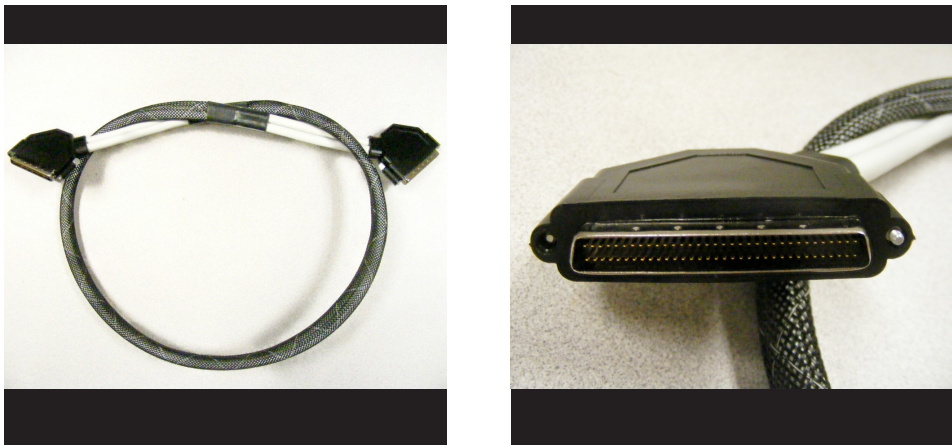
Figure 3-4 DS1 Signal Cable and Connector
