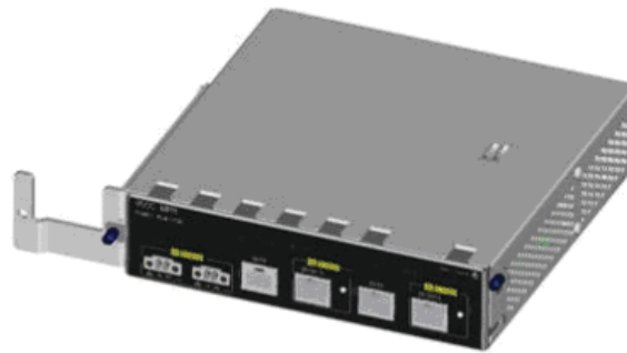
Figure 57. Power Injector box
