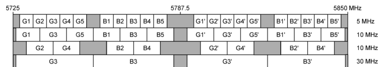
Figure 3.66 – Frequency plan 9558HC: 5.725 to 5.850 GHz unlicensed band (FCC Part 15 and IC RSS-210)
