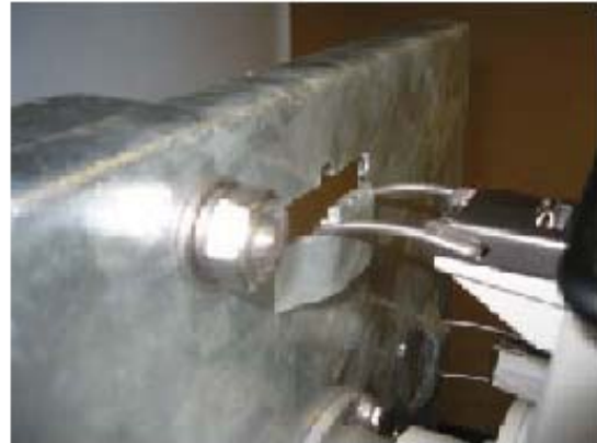
Figure 528. MPT-MC 1+0 installation for not integrated antenna (with pole mounting P/N 3DB 10137 AAAB)
