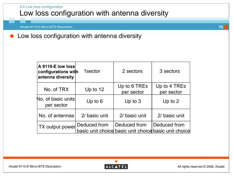
■ The exact number of antennas depends on the use of panel/ cross-polarized/integrated antennas.
