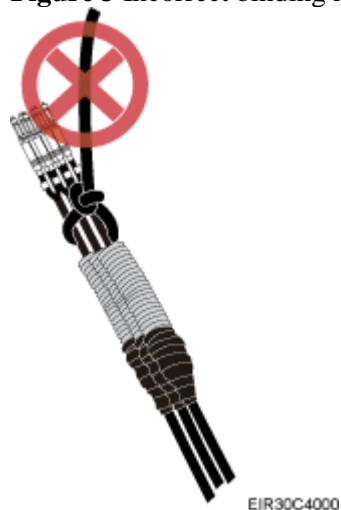
Figure 3 Incorrect binding method
