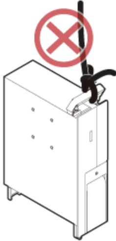
Figure 3 Incorrect binding method (1)
