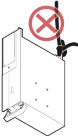
Figure 4 Incorrect binding method (2)
