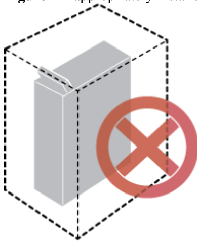
Figure 1 Inappropriately installed RRU
