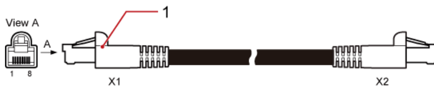
Figure 7-28 FE surge protection transfer cable
