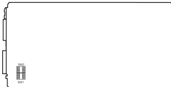
Figure 3-16 Positions of DIP switches on the UMPT
