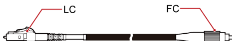
Figure 7-31 FE/GE fiber optic cable (with the FC and LC connectors)
