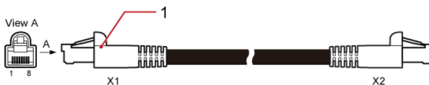
Figure 7-43 ELU signal cable
