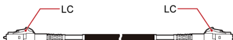
Figure 7-33 FE/GE fiber optic cable (with the LC connectors)
