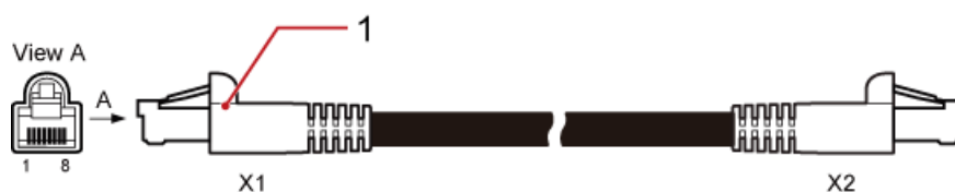
Figure 7-29 Interconnection cable between FE electrical ports
