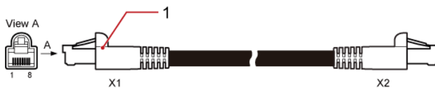
Figure 7-42 BBU alarm cable
