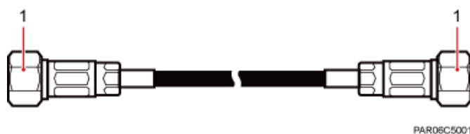
Figure 7-48 RRU RF jumper
