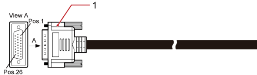
Figure 7-25 E1/T1 signal cable
