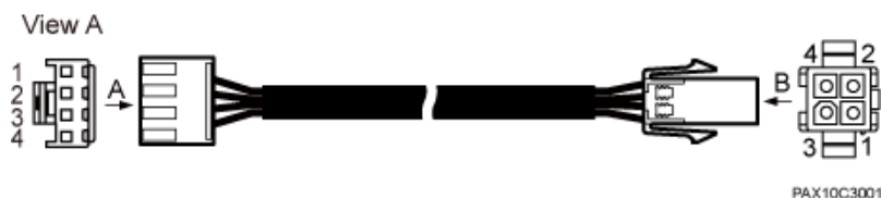
Figure 7-38 Monitoring signal cable for the fan assembly
