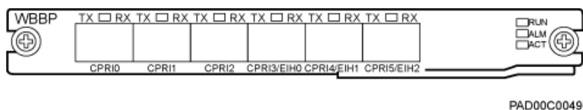
Figure 3-22 Panel of the WBBPd
