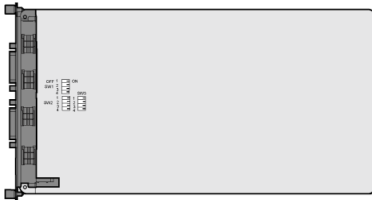
Figure 3-44 DIP switches on the UTRPb4
