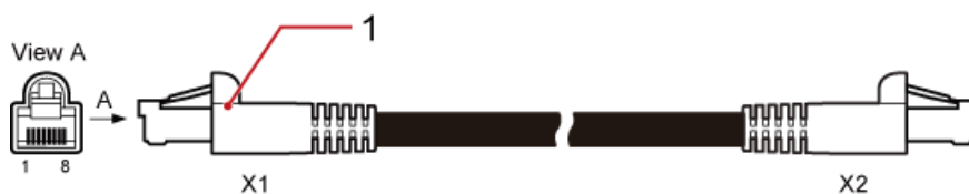
Figure 7-27 FE/GE Ethernet cable
