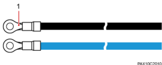
Figure 7-18 DC input power cable for the BTS3900C
