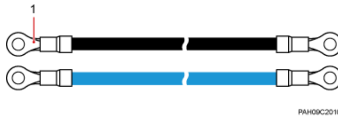
Figure 7-21 PDU10D-01 power cable
