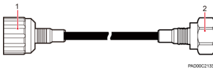
Figure 3-5 Exterior of an RU RF jumper (1)
