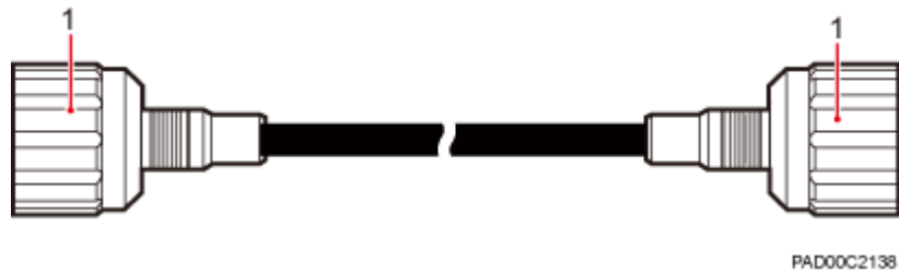
Figure 3-6 Exterior of an RU RF jumper (2)
