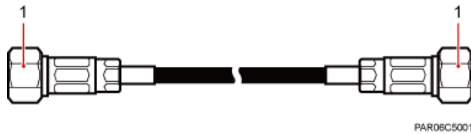
Figure 3-4 Exterior of an RRU/RFU RF jumper
