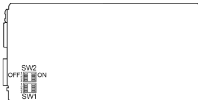
Figure 2-78 Positions of DIP switches on a UMPTa series board
