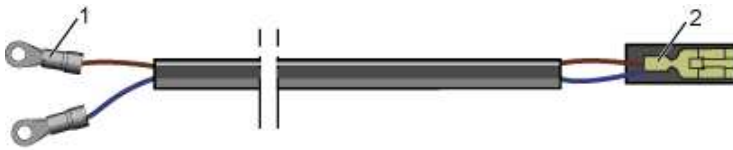
RRU3908 – 48V external input power cable
