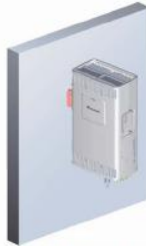
Installation on the wall (flag mode)
