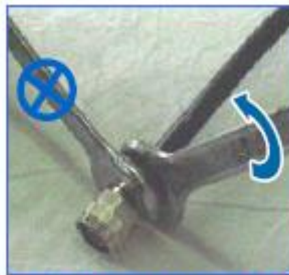
Fasten the body and crimp
