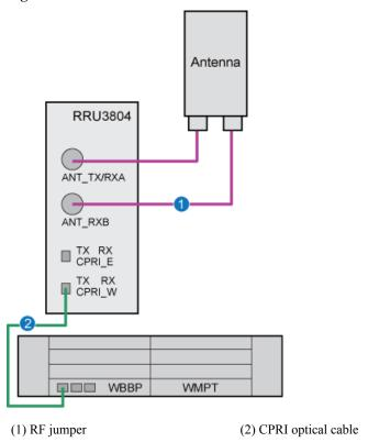
Figure 4-7 Cable connections of the BTS3900C in 1x3 configuration
