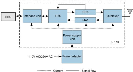
Figure 3-7 Logical structure of the pRRU3801 with optical ports
