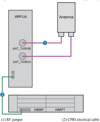
Figure 4-16 Cable connections of the NodeB supporting 2x2 MIMO (WRFUd configured)
