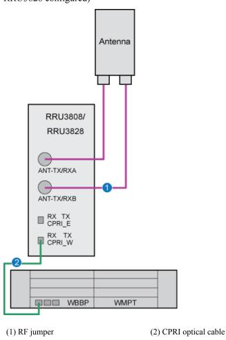
**Figure 4-14** Cable connections of the NodeB supporting transmit diversity (RRU3808, or RRU3828 configured)
