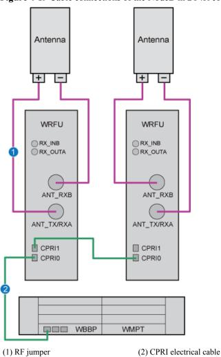
Figure 4-19 Cable connections of the NodeB in 2T4R configuration (WRFU configured)
