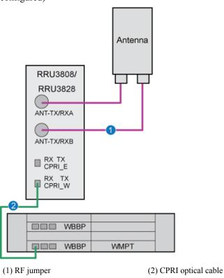
**Figure 4-6** Cable connections of the NodeB in 3x4 configuration (RRU3808, or RRU3828 configured)
