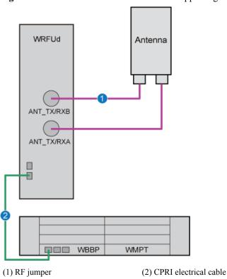
Figure 4-12 Cable connections of the NodeB supporting transmit diversity (WRFUd configured)
