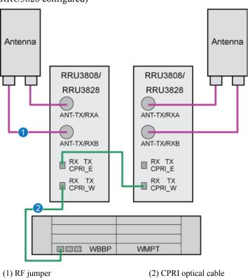
**Figure 4-10** Cable connections of the NodeB supporting 4-way receive diversity (RRU3808, or RRU3828 configured)
