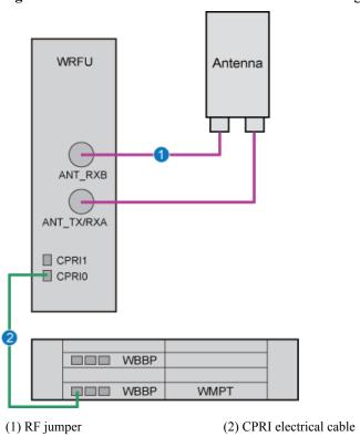
Figure 4-2 Cable connections of the NodeB in 3x4 configuration (WRFU configured)
