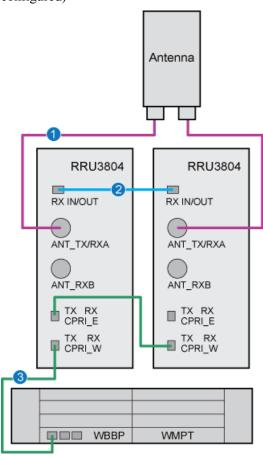
**Figure 4-17** Cable connections of the NodeB in 2x2 MIMO configuration (RRU3804 configured)
