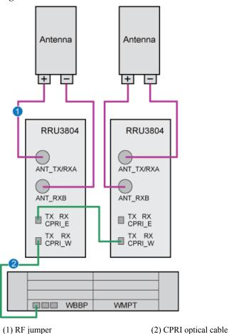
Figure 4-20 Cable connections of the NodeB in 2T4R configuration (RRU3804 configured)
