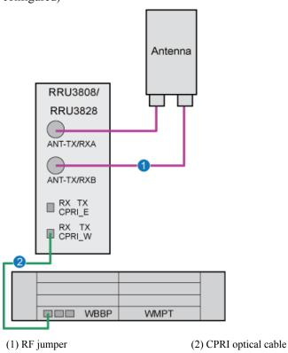
**Figure 4-5** Cable connections of the NodeB in 3x1 configuration (RRU3808, or RRU3828 configured)
