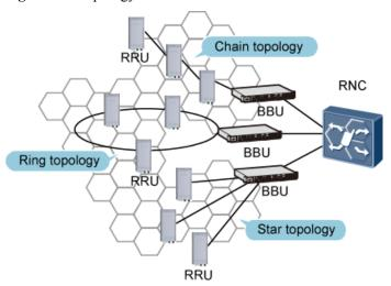
Figure 6-5 Topology between the BBU3900 and the RRUs
