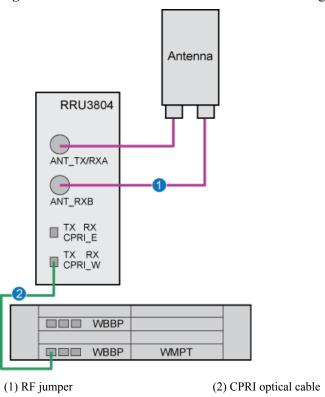
Figure 4-4 Cable connections of the NodeB in 3x4 configuration (RRU3804 configured)
