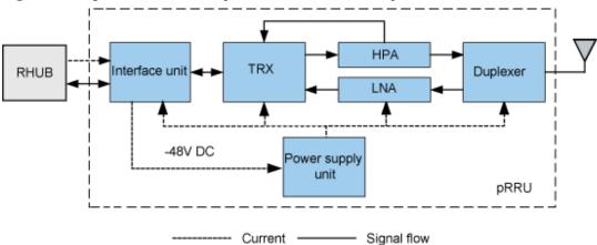
Figure 3-8 Logical structure of the pRRU3801 with electrical ports
