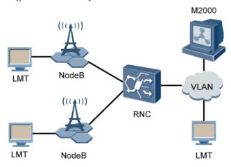
The OM subsystem of the NodeB consists of the following components:
