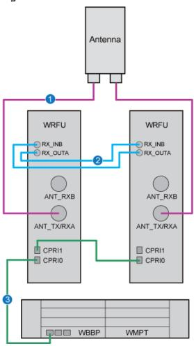
Figure 4-15 Cable connections of the NodeB in 2x2 MIMO configuration (WRFU configured)
