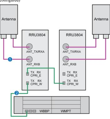
**Figure 4-9** Cable connections of the NodeB supporting 4-way receive diversity (RRU3804 configured)
