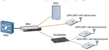
Figure 6-9 BBU3900, RRU, and pRRU in the hybrid topology
