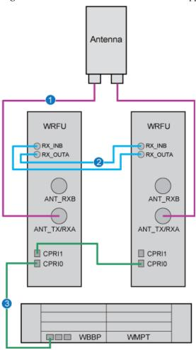
Figure 4-11 Cable connections of the NodeB supporting transmit diversity (WRFU configured)
