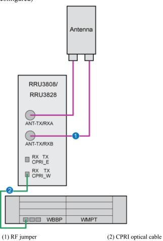
**Figure 4-18** Cable connections of the NodeB supporting 2x2 MIMO (RRU3808, or RRU3828 configured)
