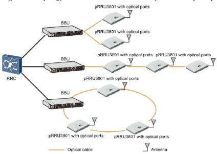
Figure 6-7 Topology between the BBU3900 and the pRRU with optical ports
