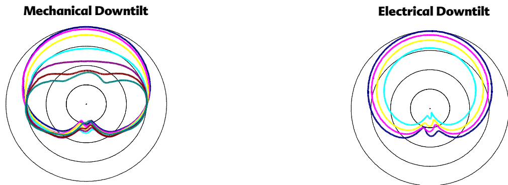
Radiation intensity does not change at 90 degrees
