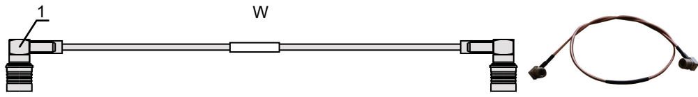
Figure 5-27 Inter-DRFU RF signal cable
