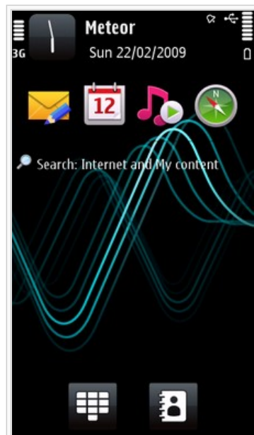
S60 5th edition idle screen. Bottom left "button" brings up a virtual number pad, to compensate for removal of actual numerical keys.
